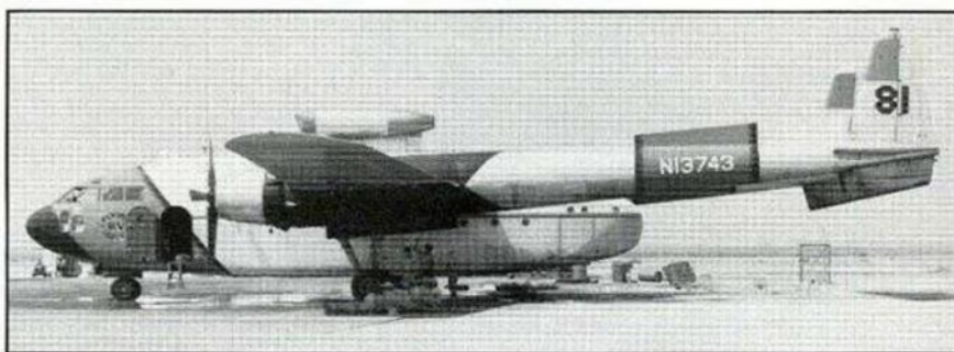
Top: A Douglas A26 Invader drops 5000 litres of retardant slurry mixture on burning timber at a sawmill in Minnesota, USA. Above: A Fairchild C119 Flying Boxcar tanker. Twenty of these former military transports, fitted with an auxiliary J34 turbo-jet engine to improve take-off performance, have been converted for use as fire-bombers.
