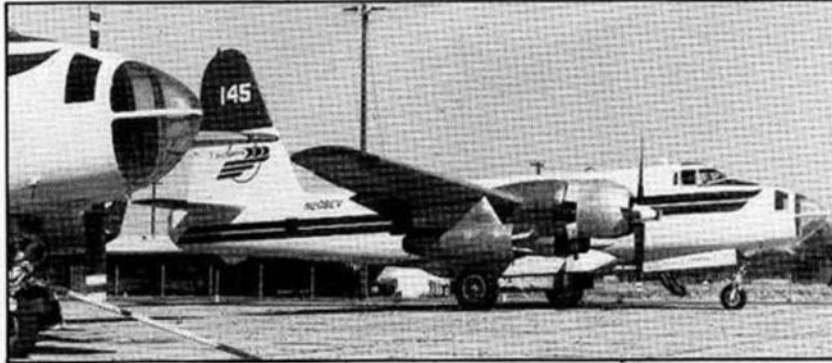
Top: Among the biggest fire-bombers operating in the U.S. today are former airline DC7s — able to drop 13,000 litres of retardant. Above: A pair of Lockheed P2V-7 Neptune tankers. Several operators have converted this type into successful fire bombers. Below: A line-up of DC7 tankers parked for the winter at the home base of an Arizona fire bomber company.
